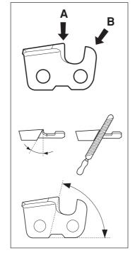
It is very difficult to sharpen a chain correctly without the right equipment. We recommend you to use a file gauge. This will help you obtain the maximum kickback reduction and cutting performance from your chain.
